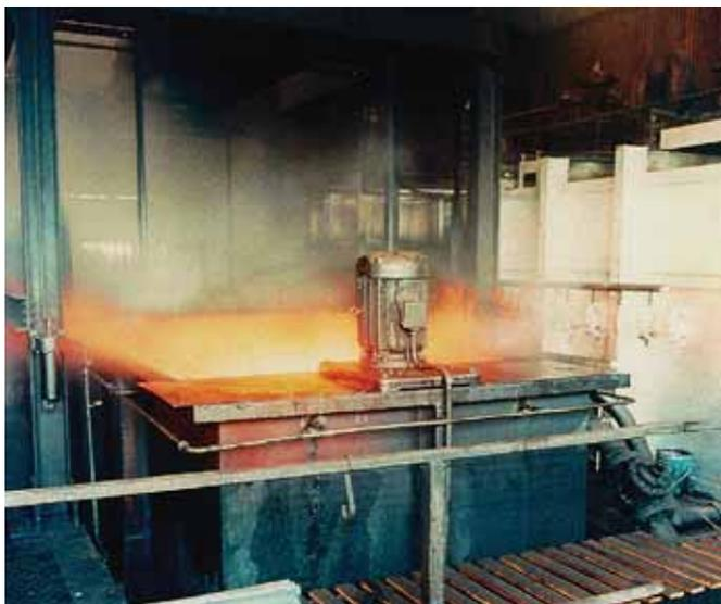
Figure 4 | Fire is a major concern in working with quenching oils. Operating temperatures in quenching should be 55 C to 83 C (130 F to 180 F) below the oil's flash point. [Courtesy of Houghton International, Inc.]
