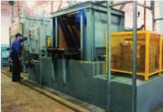
Figure 6 | Intensive quenching can be done in the 6,000-gallon system shown. (Courtesy of IQ Technologies, Inc.)
