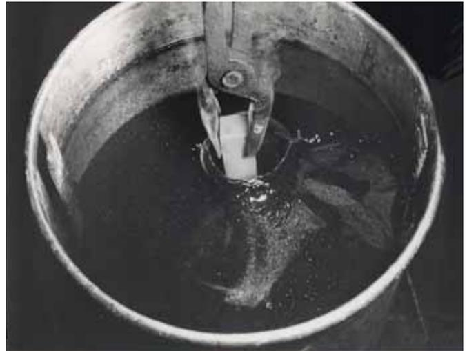
Figure 2 | Immersion of a hot piece of steel in water can generate a large vapor blanket in Stage A of the quenching process. (Courtesy of G.E. Totten & Associates, LLC)
