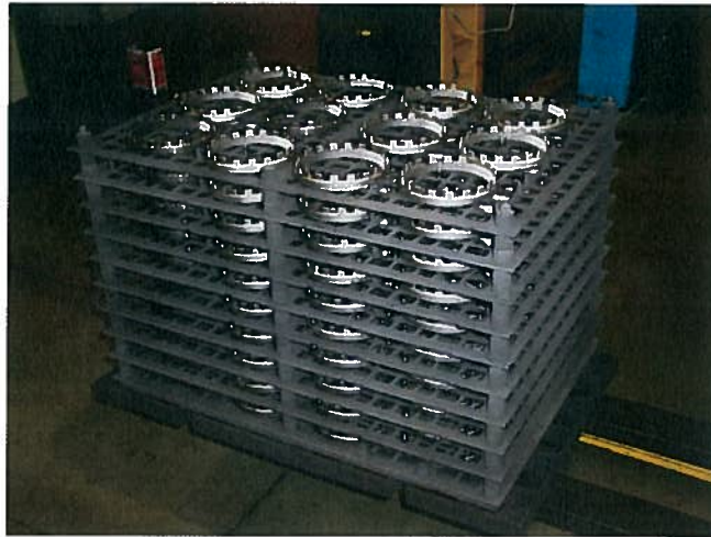
Fig. 4: CFC-fixturing for internal ring gears
